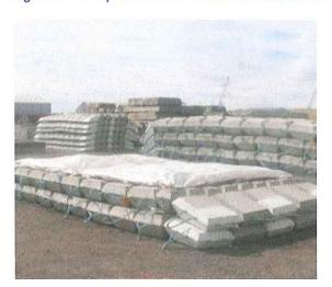
Figure 3-1 Examples of standard concrete mattresses
